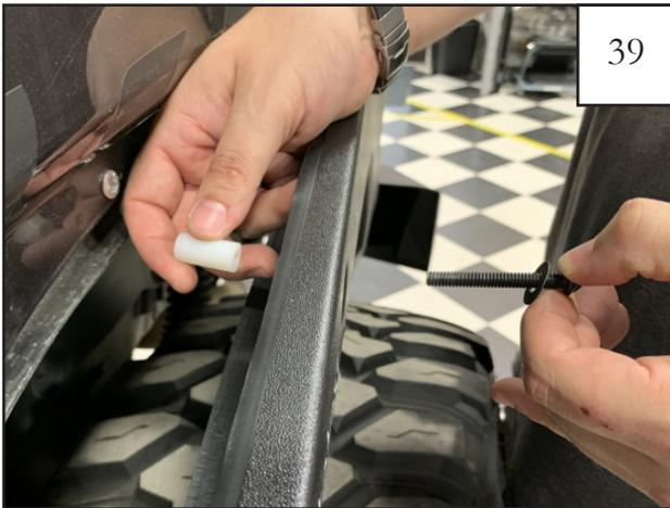
39 Install rear fender delete using 5 long bolts,(133606G) 5 washers (WA1-0029), and 5 spacers (1 short SP1-0004, and 4 long SP1-0005).
