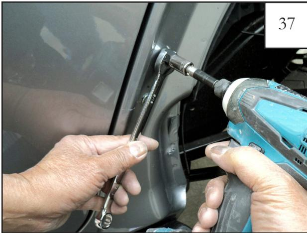
37 Using a wrench to hold rivnut tool in place, install rivnut in place on fender using an 11/16" socket. The rivnut will expand to secure itself in place. NOTE: Use of impact driver recommended for rivnut installation.
