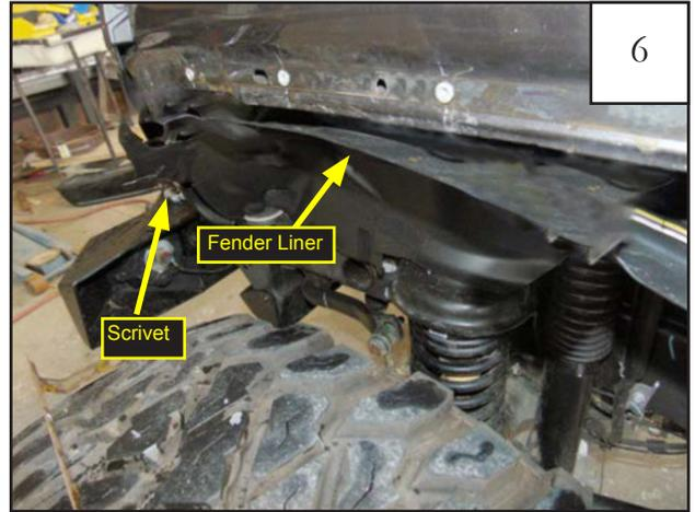
Reinstall the splash shield using the previously removed factory scrivet in preparation for marking before cutting.
