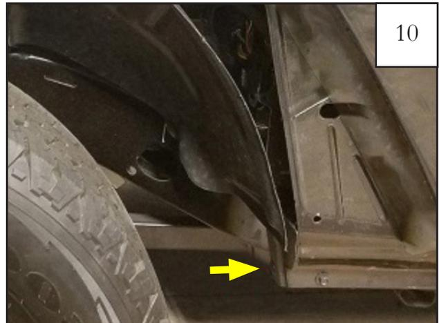
**NOTE:** It may be necessary to trim the factory installed lower plastic cover piece indicated above to obtain correct fit.
