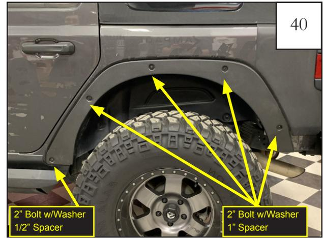
40 Use the noted hardware combinations to install the fender delete. Install from rear to front loosely. Tighten bolts once all 5 are installed.
